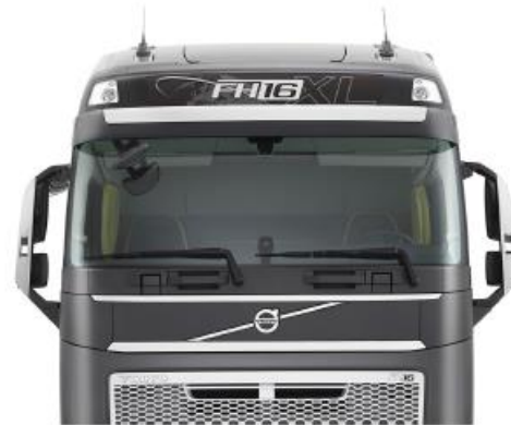
Camera in the upper centre area of the windscreen.
