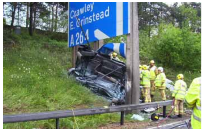
Figure 17: This photograph from the UK shows the unfortunate consequences of hitting a solid sign structure. Note the rigid crash barrier is also a hazard.
