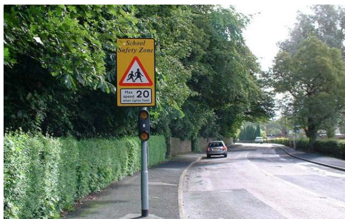
Figure 13 – example of a special school safety zone sign from the UK. Whilst this sign face contains additional advice for motorists, flashing lights such as these are also used in conjunction with just the 'children' symbolic triangle sign without the additional advice. (Source: Glossop, Derbyshire, UK)
