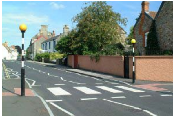
Figure 4 – zig-zag lines at a zebra crossing in the UK from 2pass.co.uk website
