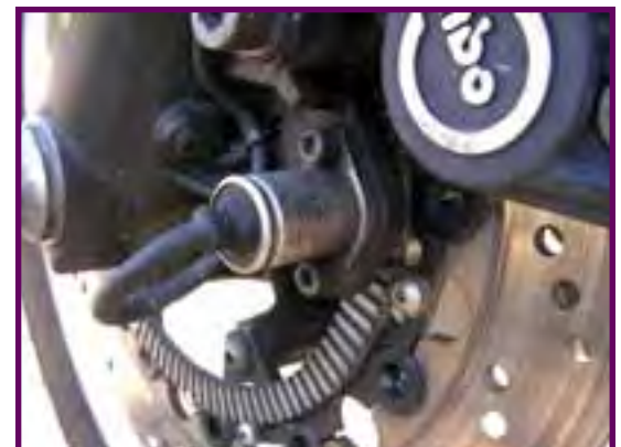
Antilock Braking System front sensor on a BMW 1100 LT motorcycle
