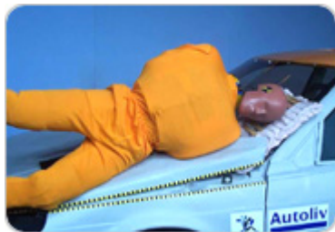
Autoliv Pedestrian Protection Airbag Source: www.autoliv.com
