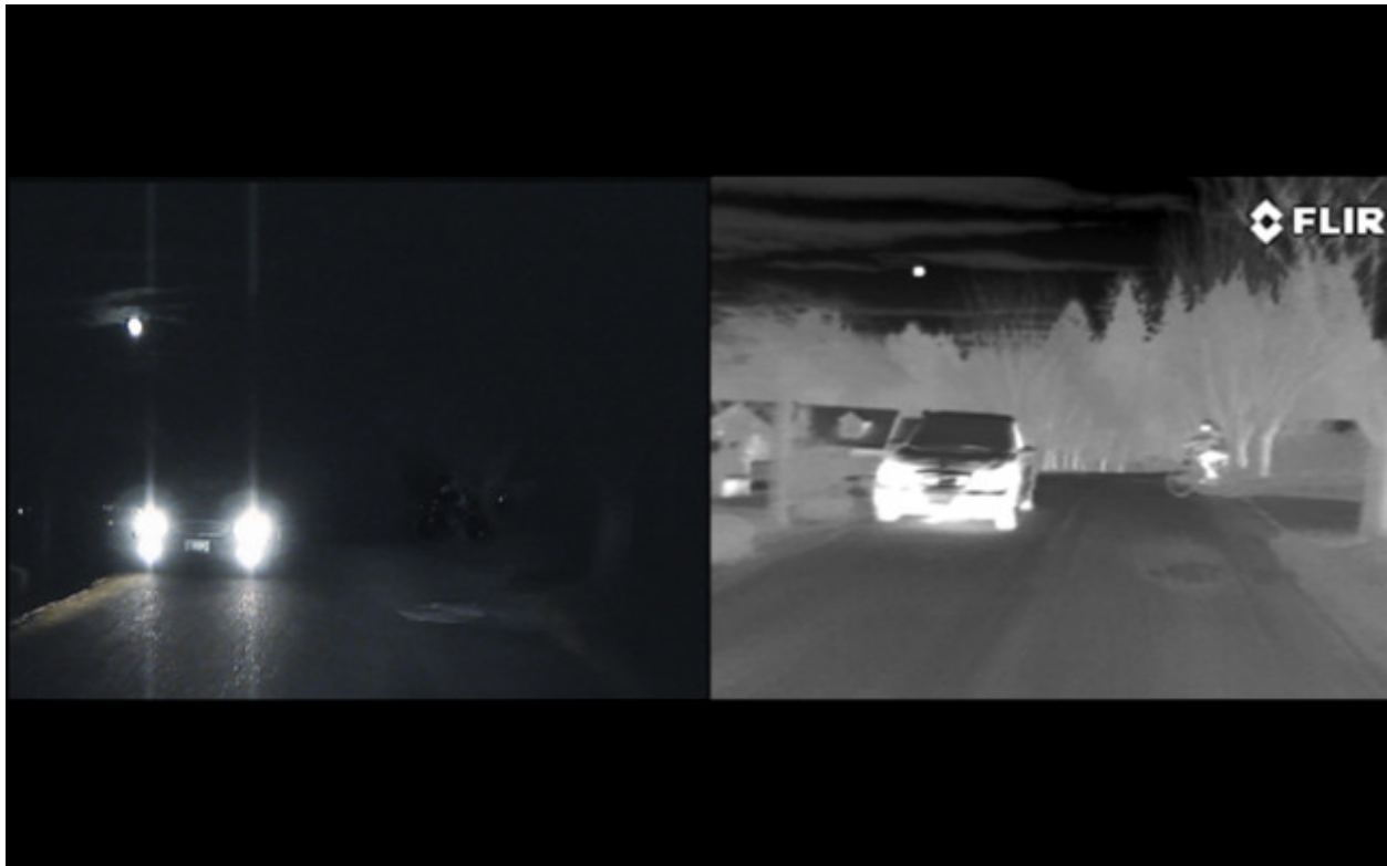
Two photos of the same scene at night of a cyclist. Standard driver view (left) and drivers view using infra red camera display (right).
