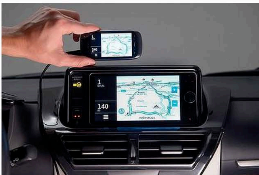
Toyota's TouchLife entertainment system will mirror a driver's smartphone on the car display
