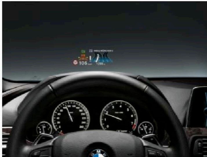
BMW 5 Series full colour heads up display includes current speed, posted speed limit, vehicle condition, lane keeping and blind spot monitoring as well as navigation information
