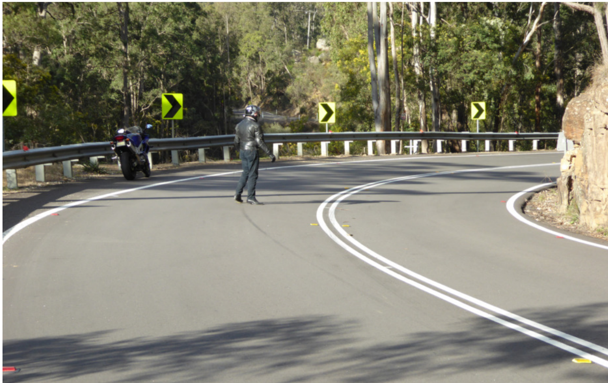
Recent improvements to Putty Road, installation of arrows. This corner was the scene of multiple crashes due to an optical illusion under certain lighting conditions that made the road look like one continuous section across the gully resulting in multiple crashes into the W Beam. (Photos, Clements)
