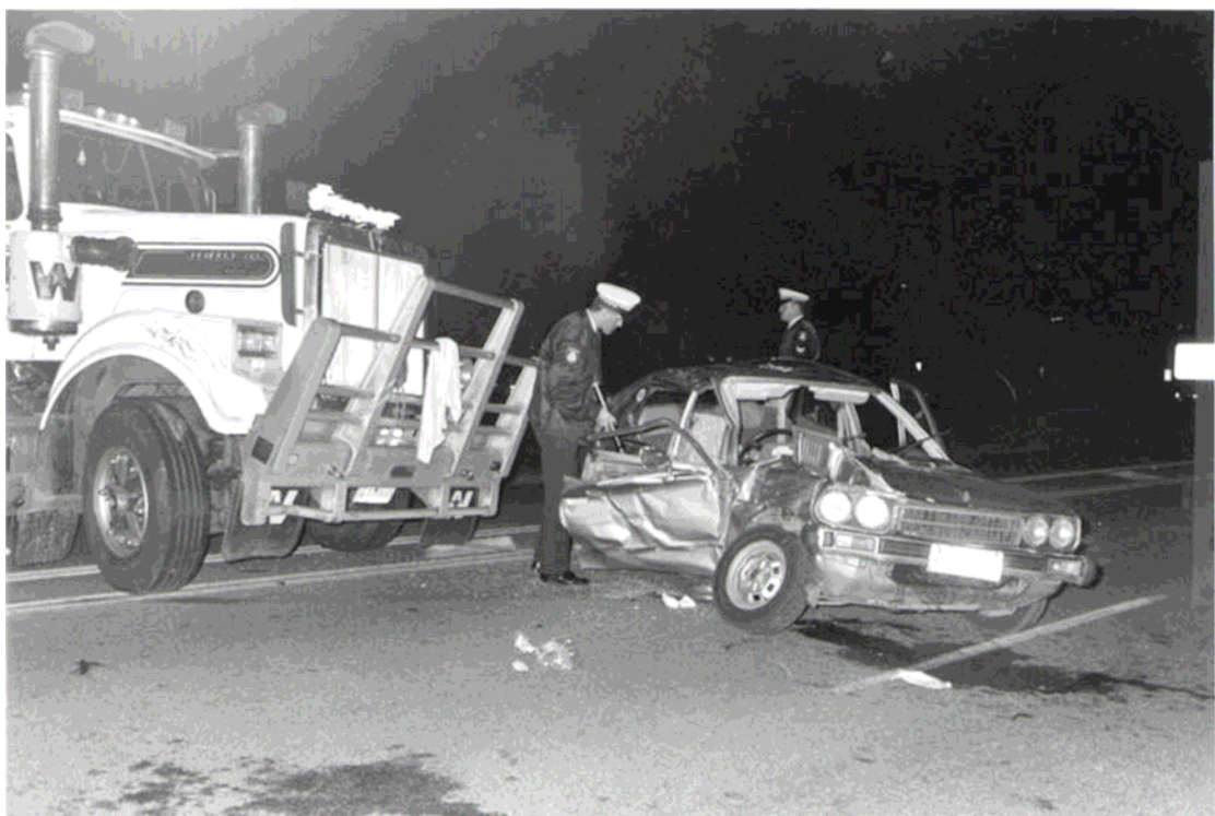
Figure 2: Over ride and hard front facia result in serious head and chest injuries. In the lower picture the occupant survival space is maintained but impact to the head of the driver results in fatal injuries.
