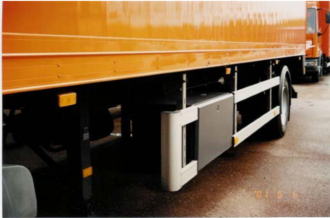
Figure 4: Side skirting to help prevent under-run in car collisions and over-ride of cyclists and motorcyclists during turning manoeuvres.
