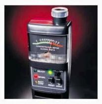
This device is a simple hand-held unit. It is powered by a set of 6 AA sized batteries, which give it sufficient power for approximately 500 breath tests.
