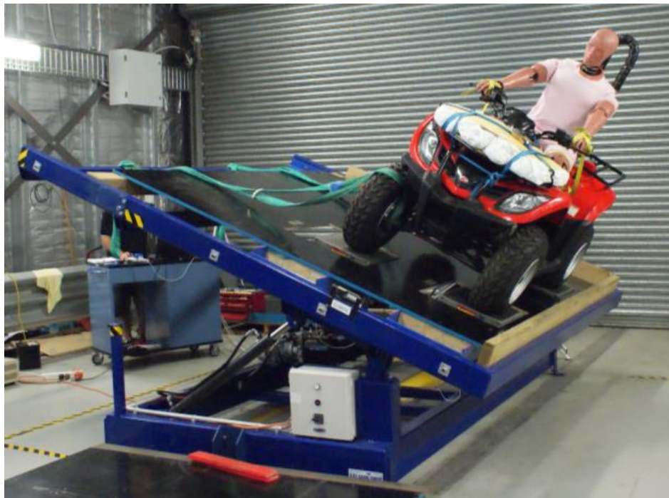
Figure 2 Quad Bike with CPD being tested for lateral roll stability
