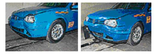
VW Golf IV–Identical deformations following AZT crash repair test on passenger vehicle in original condition (above) and following correct repairs (below).
