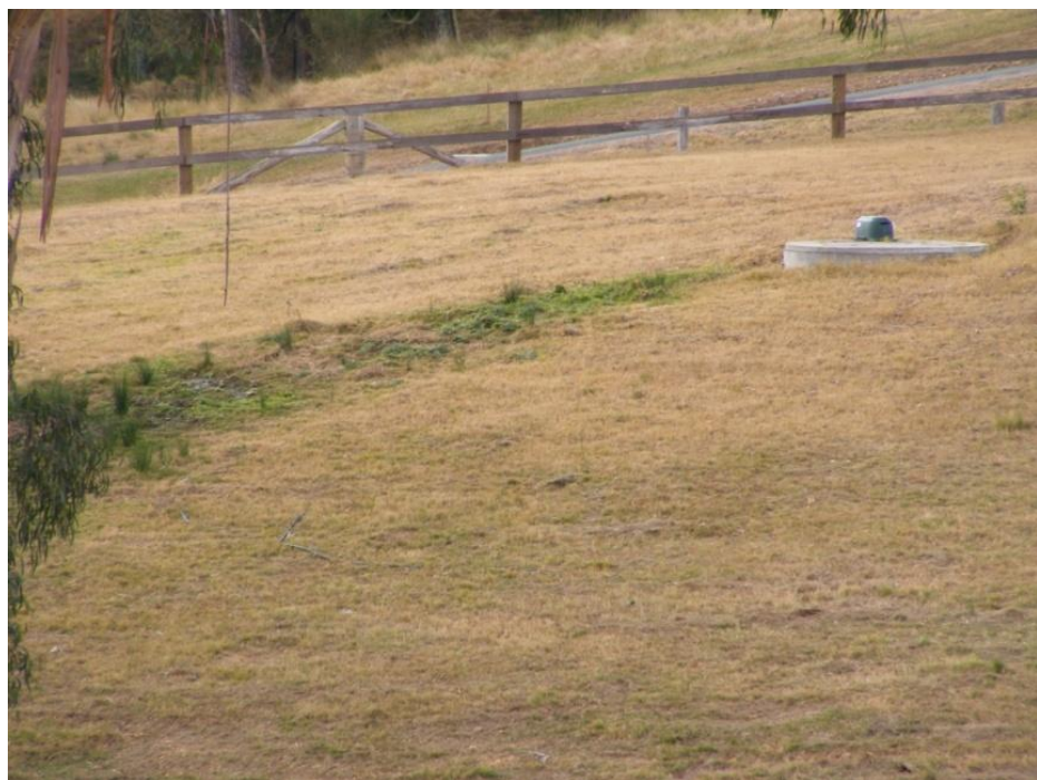
FIGURE 4: A FAILING AWTS - UNSERVICED
