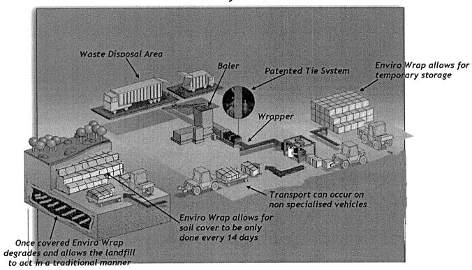
NOTE: This system can be placed at transfer stations or resource recovery facilities it does not need to be at the landfill
