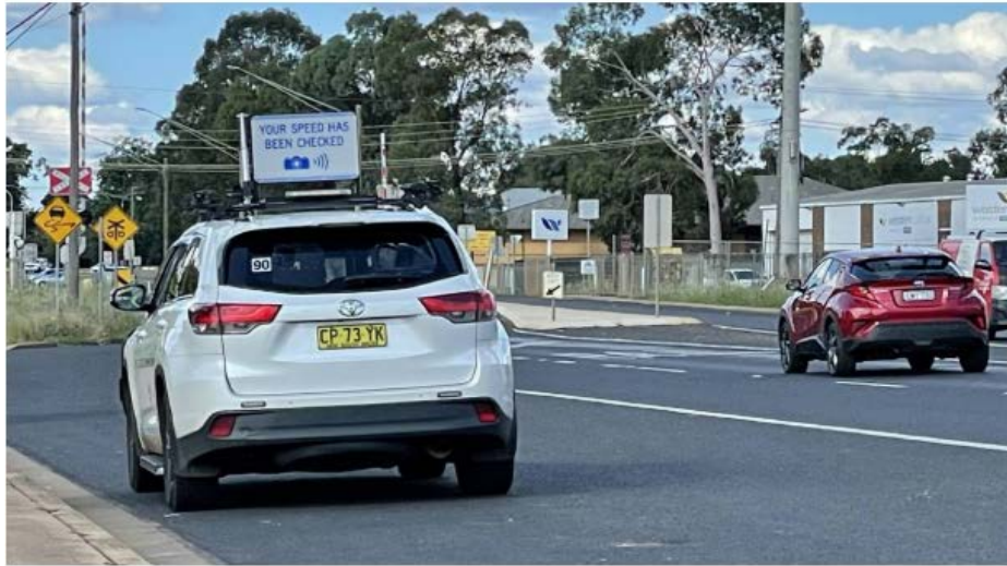
Figure 1: Retractable warning sign on detection vehicle on Cobbora Road in Dubbo 38
