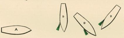
If A sees a mast-head light above the green light A knows that the vessel is a steam vessel and is either approaching her in the same direction as B or is crossing to starboard in some direction as D D D.
