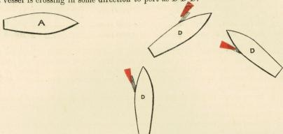
If A sees a white mast-head light above the red light A knows that the vessel is a steam vessel and is either approaching her in the same direction as B or is crossing to port in some direction as D D D.
