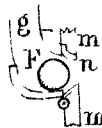
Figure 5. Section of spherical valve for horizontal vapour-pump referred to in second claim.
