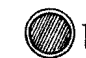
Figure 13. Section of pipe with central solid core, which may be of any solid not acted on by the contents, in order to diminish the area relatively to the surface referred to in eleventh claim.
